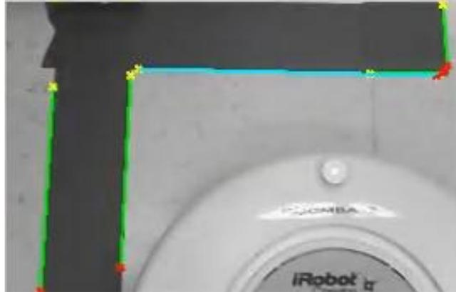
Figure 6. Processed image from the camera detecting the horizontal lines on the front and left front wall.
