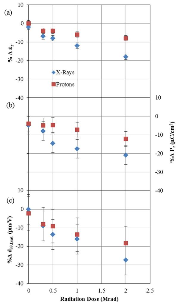
FIG. 1. Percentage change in the (a) low field dielectric permittivity, measured at 0.25 kV/cm and 1 kHz, (b) remanent polarization, measured at 1 kHz, and (c) effective saturated piezoelectric response ( $d_{33,f,sat}$ ) of the PZT thin films, measured at 10 kV/cm AC and 40 kV/cm DC fields and 1 kHz, as a function of radiation dose.
