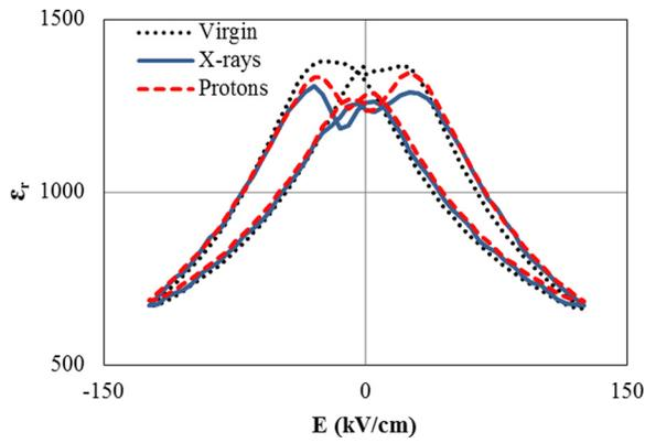
FIG. 2.  $\epsilon_r$ - $E_{DC}$  curves for a 810nm-thick PZT film, in virgin state and after irradiation by 2Mrad X rays and protons (measurements performed at 1 kHz).
