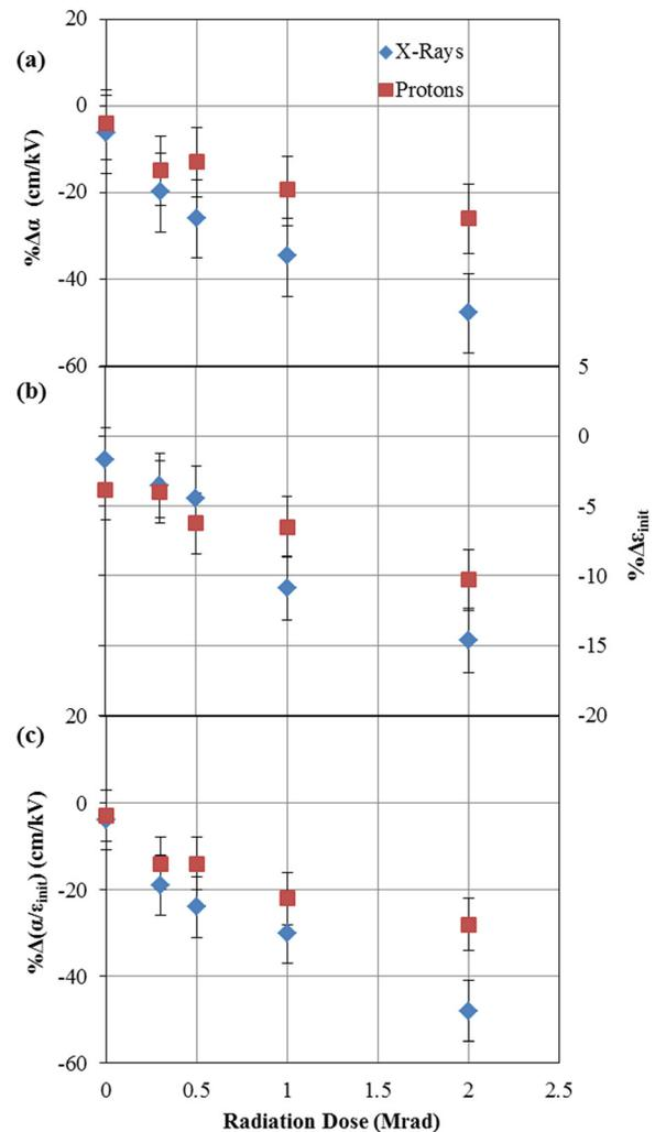
FIG. 3. Percentage changes in the (a) irreversible dielectric Rayleigh parameter,  $\alpha$ , (b) reversible dielectric Rayleigh parameter,  $\epsilon_{init}$ , and (c) the ratio of the irreversible to reversible dielectric Rayleigh parameters,  $\alpha/\epsilon_{init}$  of the PZT films measured at 1 kHz, after exposure to X rays and protons.
